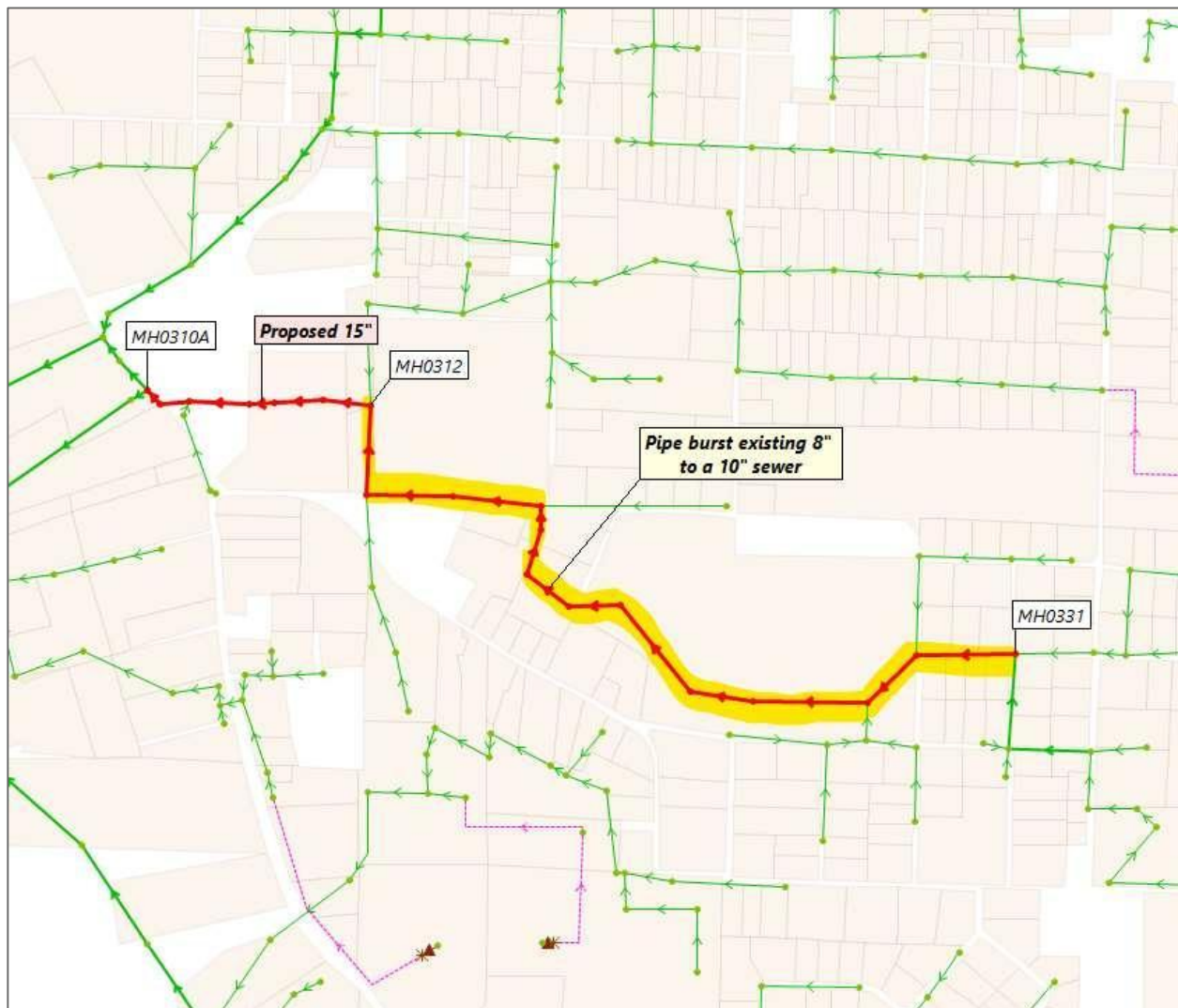
Figure 6-9. Project E – Upsizing Sewer Upstream of Sulphur Springs Road
