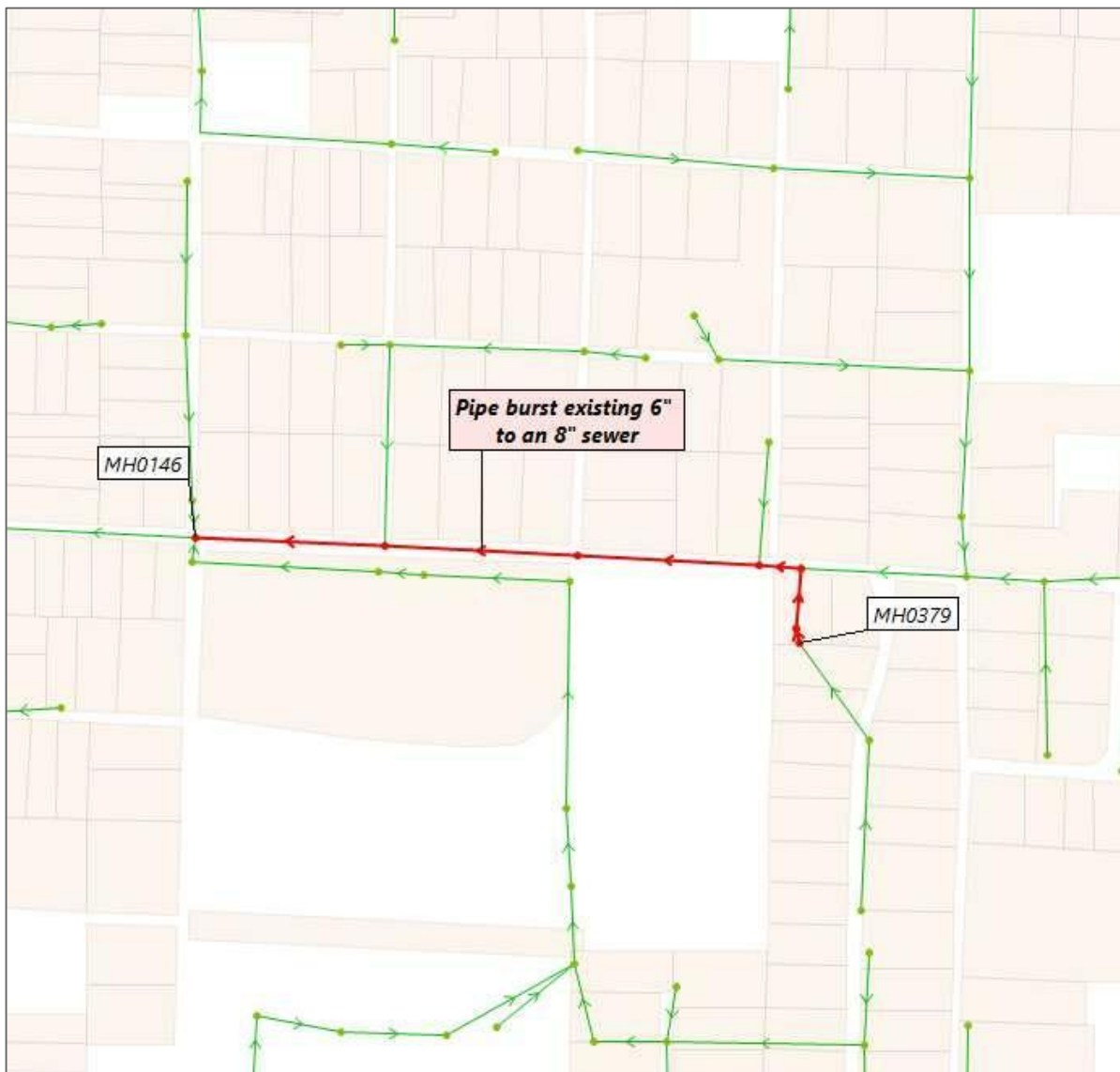
Figure 6-11. Project G – Pipe Burst Along Sullenberger Avenue
