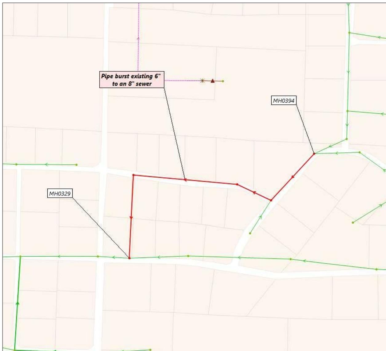
Figure 6-10. Project F – Pipe Burst at Wilson Street & Park Avenue
